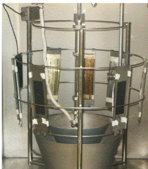
Figure 68: weatherometer with a Xenon lamp, emitting UV rays at 340 nm at an irradiance of 1.1 \text{ W/m}^2 used in an experimental tests. Source (Said, et al., 2006).
