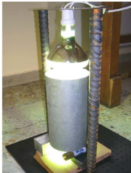
Figure 71: the experimental setup used to focus the light flux onto fibre samples.
