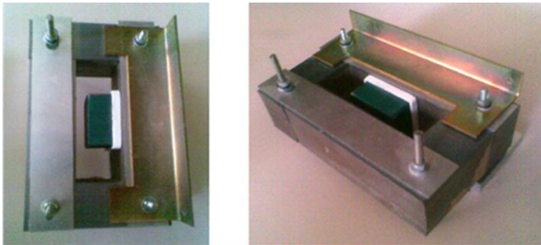
Figure 49: the homemade magnetic circuit.
