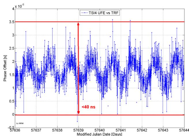
**Figure 6:** Time and Frequency Distribution via GEO Satellite: phase/time offset of the User Terminal with respect to the reference time
