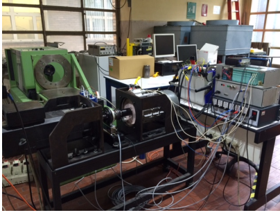
Fig. 11. Photo of test bed for magnetic model identification and efficiency measure
