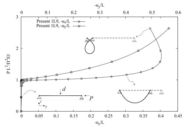
Figure 6: Post-buckling equilibrium curves of the simply-supported square cross-section beam, L/h = 100 and  $\frac{L^2}{\pi^2 EI} d = 0.004$ .
