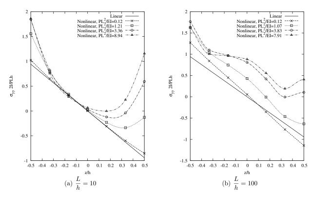
Figure 4: Through-the-thickness distribution of non-dimensional axial stress,  $\sigma_{yy} \frac{2I}{PLh}$ , on the clamped cross-section of the cantilever beam subjected to vertical loading; 1L9 model.
