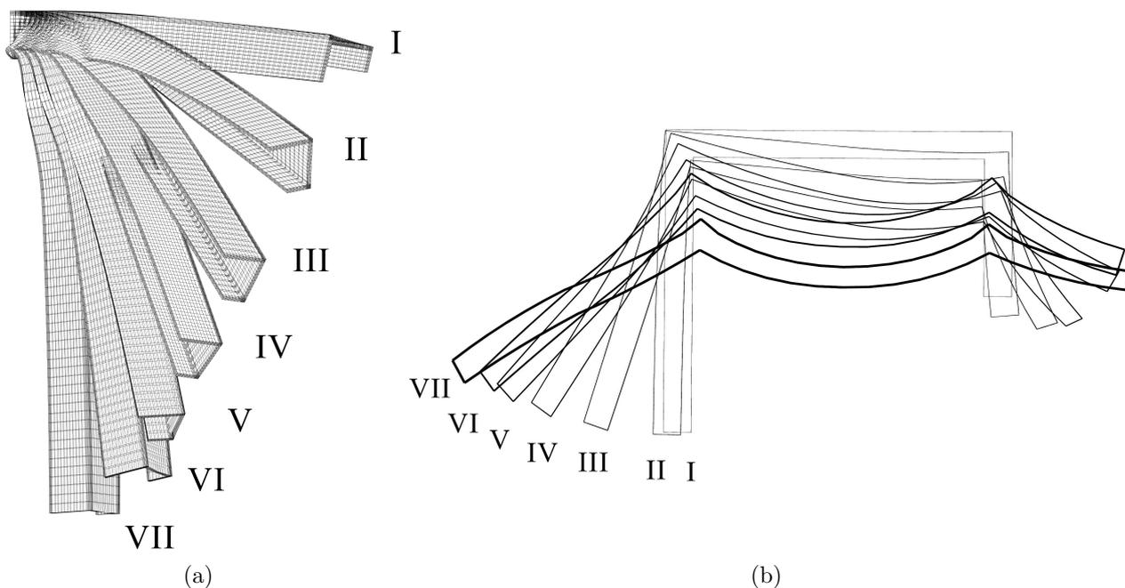
Figure 13: Three-dimensional deformed configurations (a) and cross-sections at  $y = 0.1$  m (b) for various load steps  $P = [9.52, 31.50, 40.74, 51.00, 62.62, 84.21, 192.51]$  kN. Unsymmetric C-section beam, 7L9 model.
