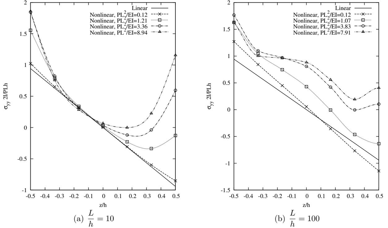
Figure 4: Through-the-thickness distribution of non-dimensional axial stress,  $\sigma_{yy} \frac{2I}{PLh}$ , on the clamped cross-section of the cantilever beam subjected to vertical loading; 1L9 model.
