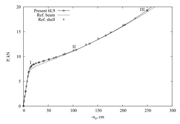
Figure 8: Equilibrium curves of the symmetric channel-section beam. Reference solutions from [27].
