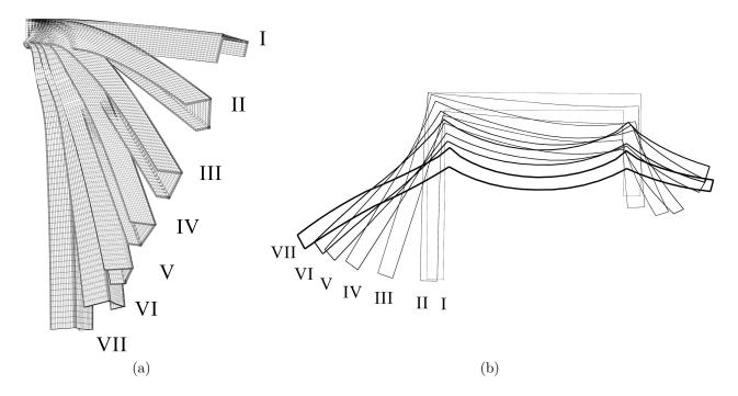
Figure 13: Three-dimensional deformed configurations (a) and cross-sections at y = 0.1 m (b) for various load steps P = [9.52, 31.50, 40.74, 51.00, 62.62, 84.21, 192.51] kN. Unsymmetric C-section beam, 7L9 model.
