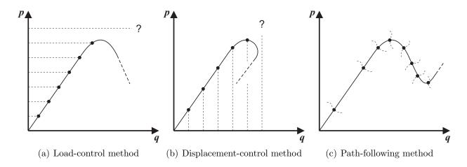
Figure 1: Representation and meaning of the constraint governing equation,  $c(\delta \mathbf{q}, \delta \lambda)$ , see [55].
