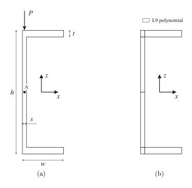
Figure 7: Cross-section geometry (a) and related 6L9 LE model subdomains discretization (b) of the symmetric channel-section beam.
