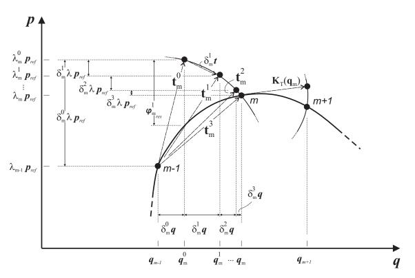
Figure 2: Geometry and notation in the incremental scheme.
