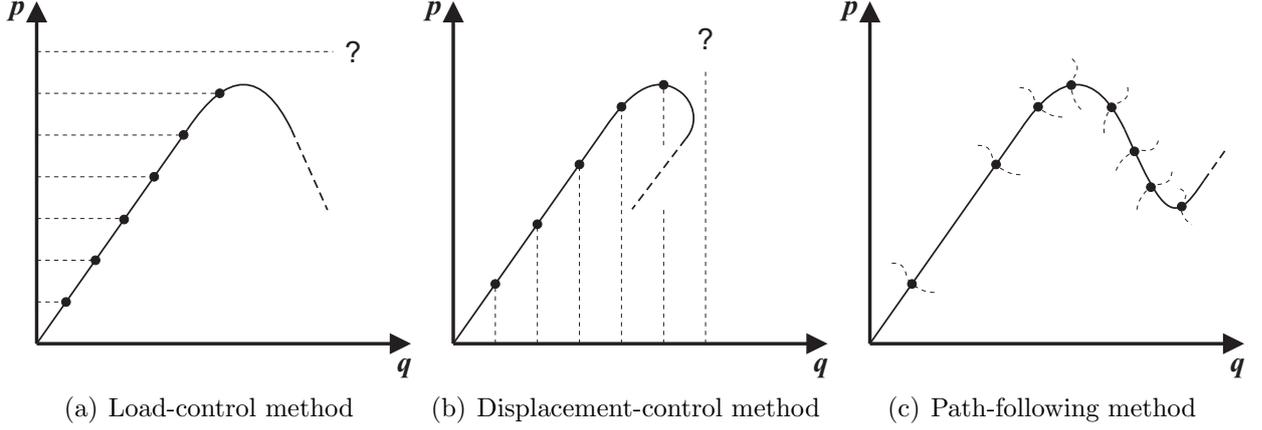
Figure 1: Representation and meaning of the constraint governing equation,  $c(\delta \mathbf{q}, \delta \lambda)$ , see [55].
