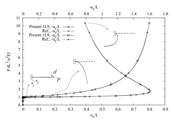
Figure 5: Post-buckling equilibrium curves of the cantilever square cross-section beam, L/h = 100 and  $\frac{4L^2}{\pi^2 EI}d = 0.002$ . Reference solution from [64].
