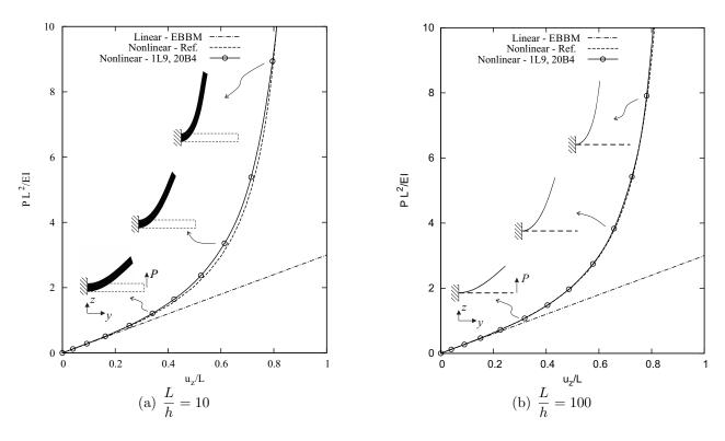
Figure 3: Equilibrium curves of the square cross-section beam subjected to vertical loading. Reference solution from [5].
