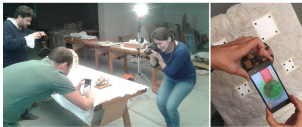
Figure 1. Acquisition phase done with different instruments: Digital Cameras used to prepare image dataset (SfM), on the right; SONY ZX1 smartphone used with the 3D Creator app, on the left.
