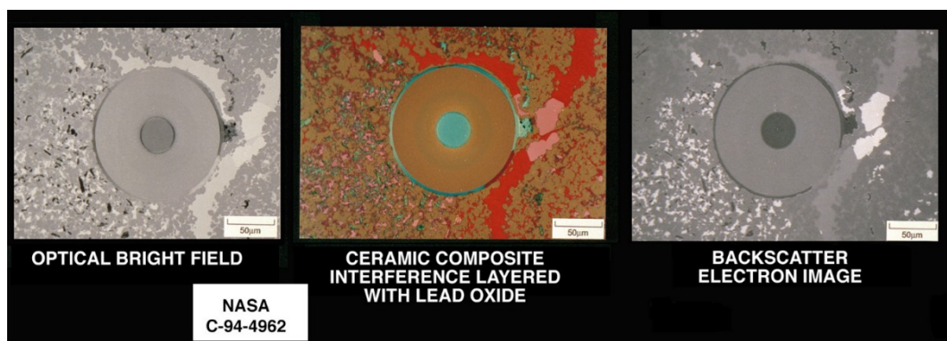
Figure 1: Thanks to the images provided by the NASA/Glenn Research Center, we can see a micrograph obtained by means of the interference layer microscopy. On the left, it is shown the specimen in an optical bright field microscopy. In the middle, we have the specimen, interference layered with lead oxide. Finally, on the right, we see a backscatter electron image.
