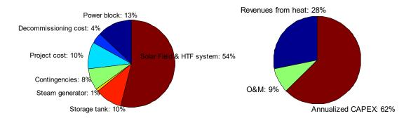
Figure 11. Left: Breakdown of the annualized investment costs, Right: Breakdown of LEC
