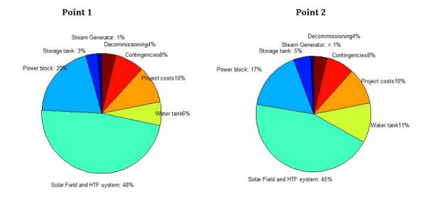
Figure13 Cost breakdown comparison between the two Pareto points selected
