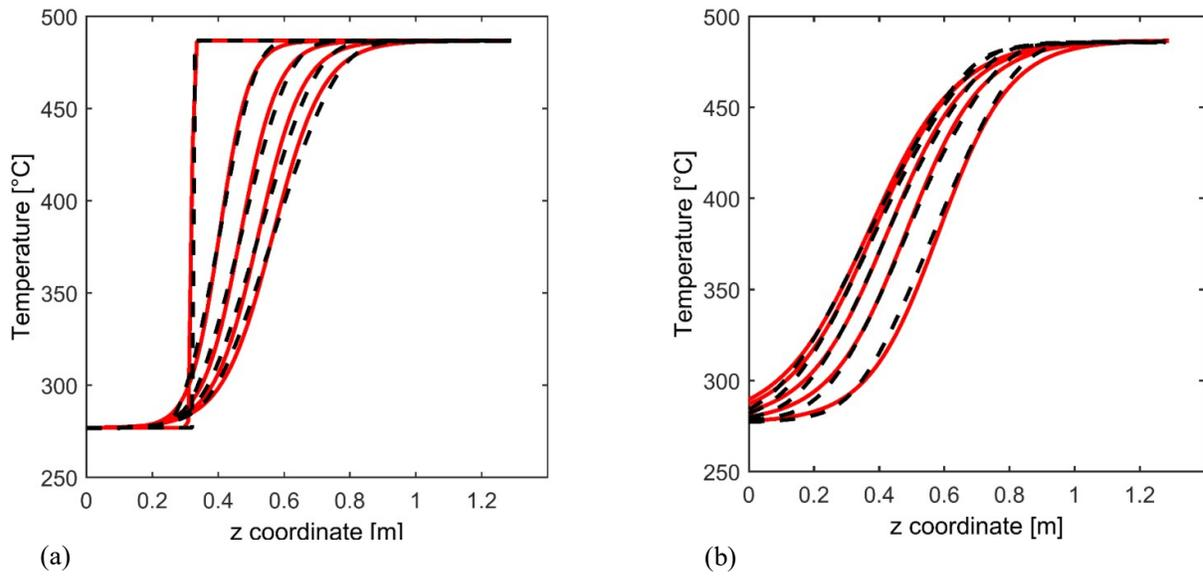
**Figure 8.** Validation of the reduced model for a continuous process with charging (a) and subsequent discharging (b) Red solid lines are the temperatures profiles obtained through the reduced model while black dotted lines are the ones obtained with the full CFD model[27].
