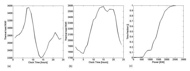
Figure 9. (a): Thermal load on the typical winter day. (b): Thermal load on the typical summer day. (c): Cumulative power distribution in the year considered.
