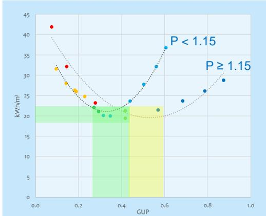
For Turin, the GUP optimal range is between 0.3 and 0.45 to ensure lowest consumptions. The presence of an optimal solar exposure allows to obtain acceptable energy consumptions also for higher GUP values.
