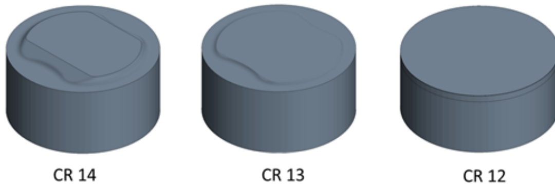
Fig. 3.25 Piston head design changes to achieve the higher compression ratio. From left to right decreasing compression ratio
