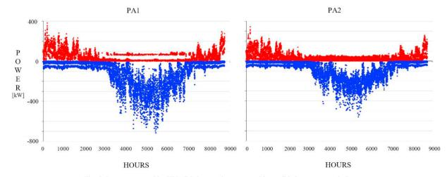
Fig. 5. Power requested by HVAC Primary Air systems with sensible heat recovery in Rome.
