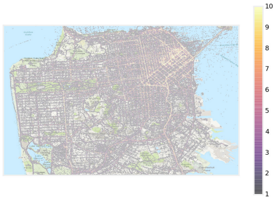
Fig. 3. Number of cells covering each location for MNO 2; lighter areas correspond to denser coverage. Maps for other operators (omitted for brevity) show a similar behavior.
