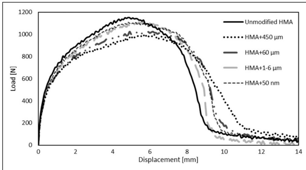
**Figure 5.** Representative load–displacement curves of the SLJ test.
