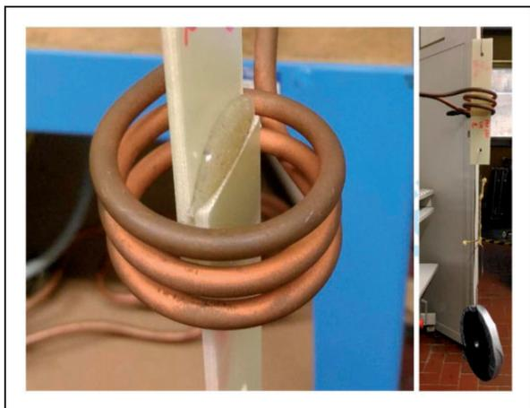
**Figure 3.** Configuration of the induction heating process.
