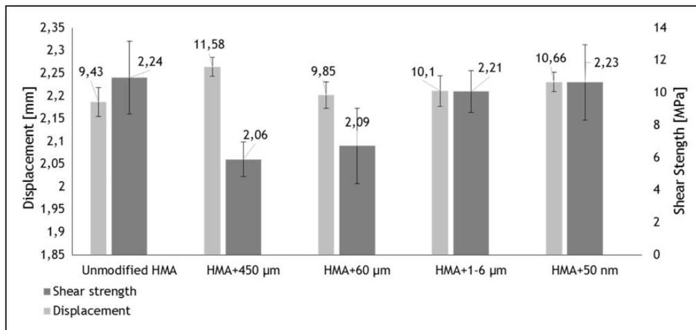
**Figure 6.** Average shear strength and maximum displacement.
