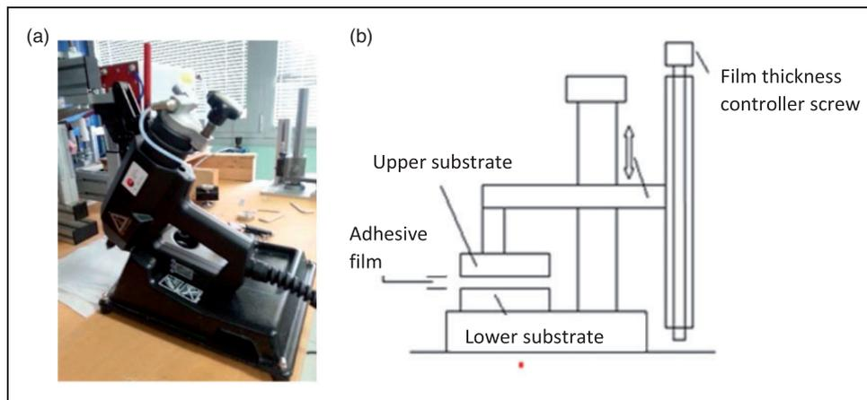
**Figure 2.** Instrumentation used for the joint preparation: (a) hot melt gun; (b) assembly device.<sup>20</sup>
