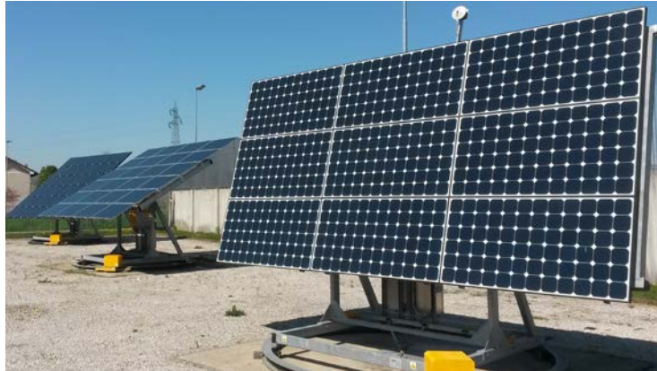
Figure 3. Example of misalignment between the plant A_{1s} (right-side of the picture) and the plants D_{1s} and E_{1s} (left-part of the picture).
