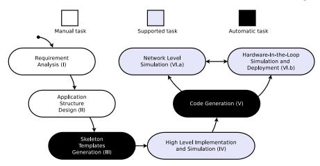
Figure 38.5: Framework development flow is based on a V-shape iterative model.
