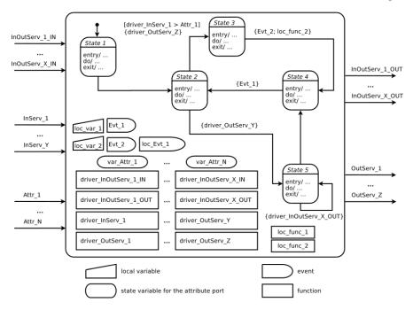
Figure 38.7: Example of complete WSN node application skeleton.
