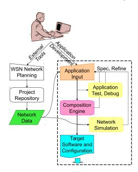
WSN network planning using specific tools for input of geographical data (e.g., of a topographic map), selection of node locations in the field, and Radio Frequency (RF) propagation simulation to estimate node connectivity.
