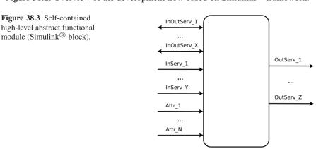
(Simulink<sup>®</sup> blocks) like the one shown in Fig. 38.3. Each module is seen as a "black box" by the other modules, being externally characterized by its tunable attributes and by the used and provided services.
