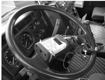
Figure 3. Adapter and measuring instrumentation fixed on a truck steering wheel.
