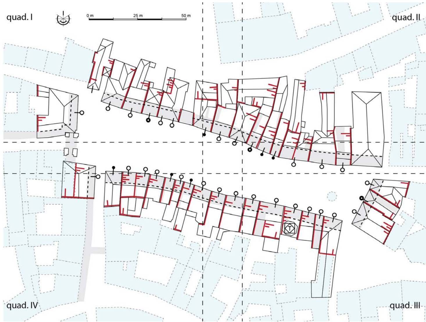
Fig. 15. Overview relative to the case study of Piazza di Santarosa – Savigliano: resistant system, geometric conformation and conditions relating to the single building and interaction between adjacent buildings forming a standardised aggregate (ref. Tab. 1 – 15). (edited by V. Donato)
