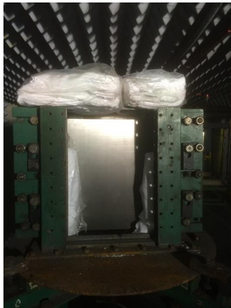
Figure 36: Target with target support and collecting cotton sheets
