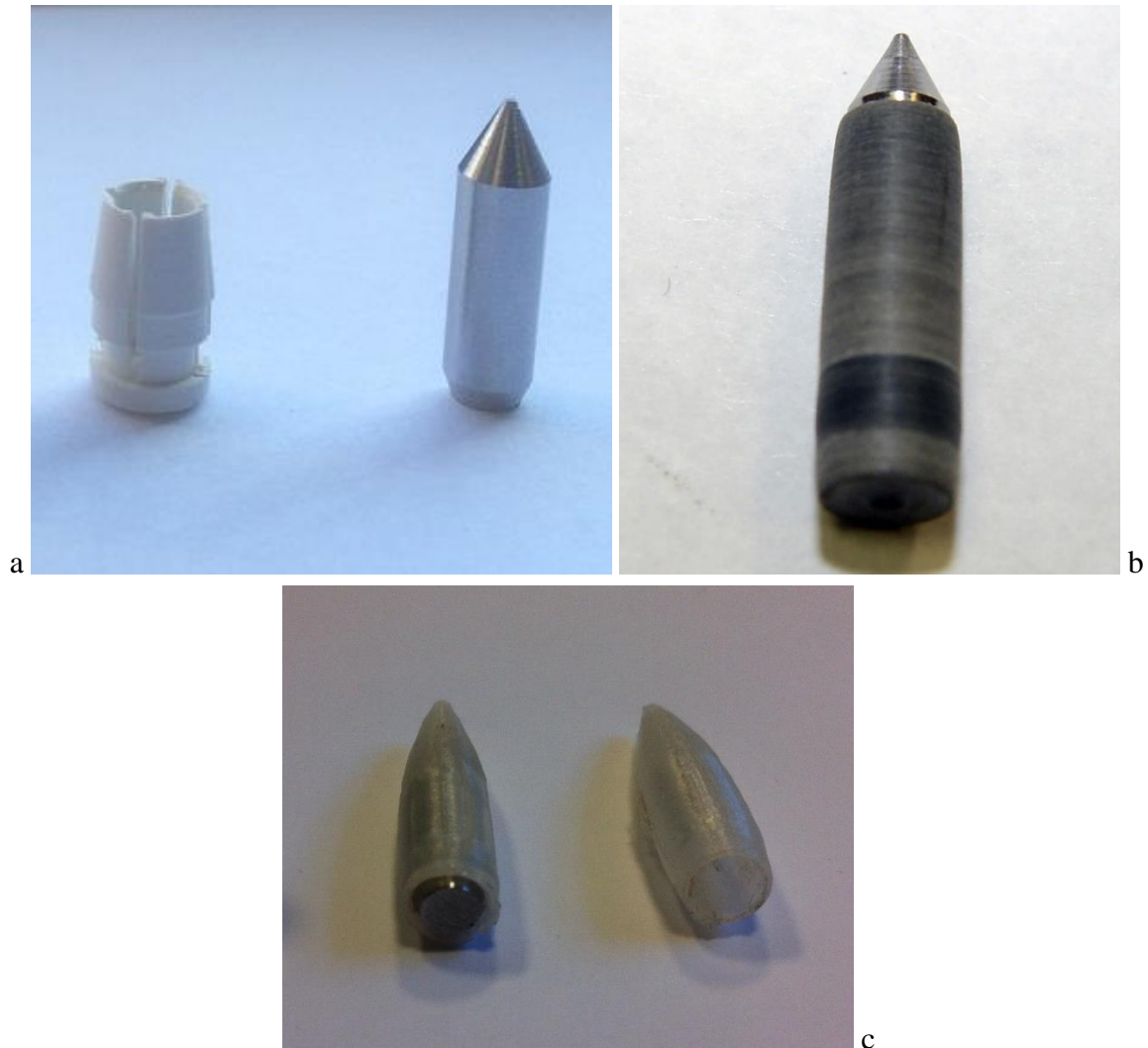
Figure 37: Plastic cases: commercial plastic sabot (a); test PVC case (b); test SLA case made by additive manufacturing
