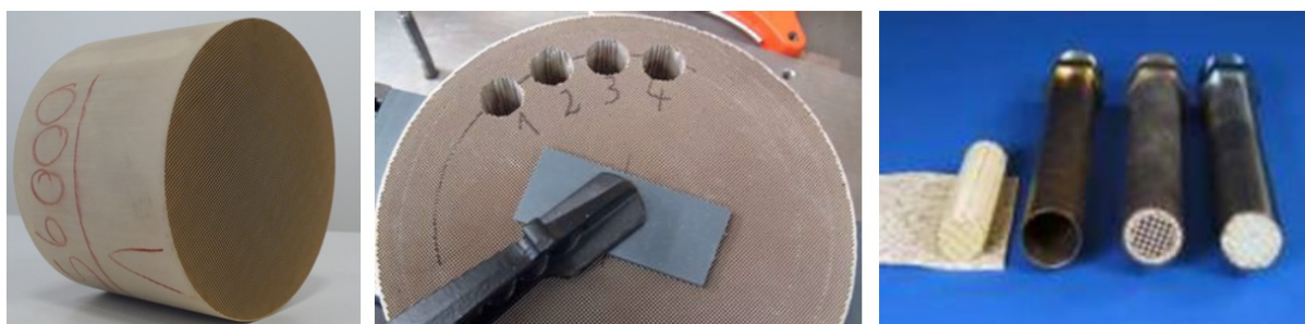
Fig. 1. Extraction of lab scale samples from full scale monolith
