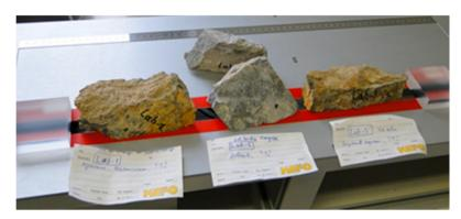
Fig. 3 Scanning of some rock samples (limestone, dolomite, marly limestone) with the TCS meter.
