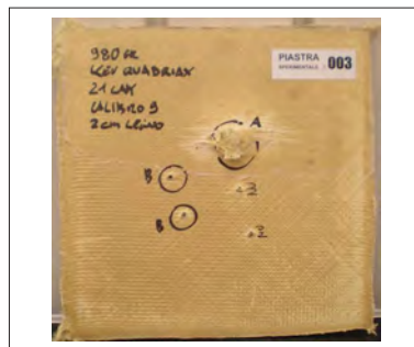
6 Ballistic test on Kevlar® composite panel: full penetration
