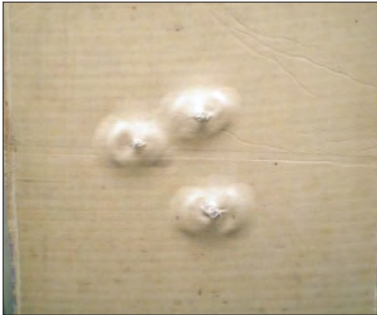
7 Ballistic test on polyethylene composite panel: no penetration with delamination visualisation
