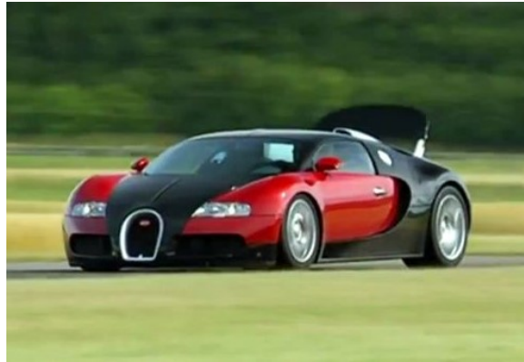
Figure 1.4 Bugatti Veyron braking using its air brake (Source: https://www.yahoo.com/news/ ).
