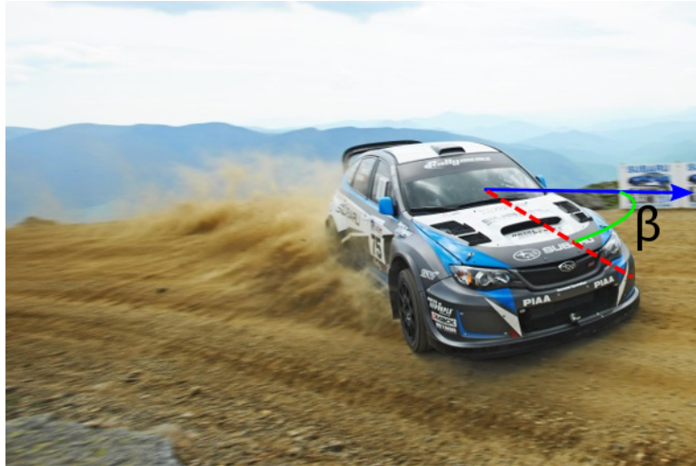
Figure 3.1 A rally driver controlling a vehicle with a large sideslip angle on a low friction road surface (Source: http://www.revvedmag.com/ ).
