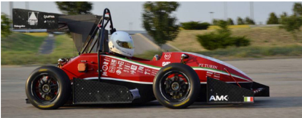
Figure 6.1 Politecnico di Torino's electric racing vehicle, the SCXV, is an AWD vehicle. It is capable of full torque vectoring due the presence of independently actuated in-wheel electric motors
