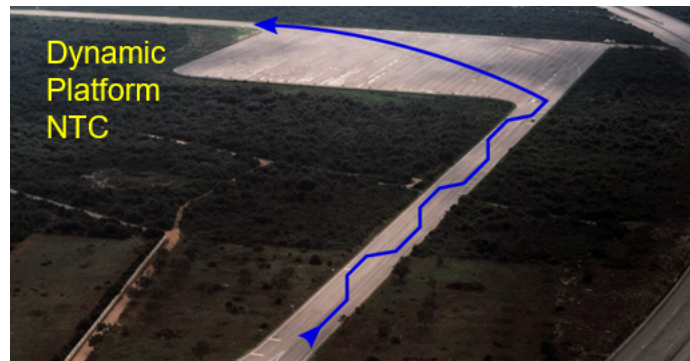
Figure 5.27 The dynamic platform at the Nardo Technical Center The dynamic platform at the NTC. This area was used for the sine sweep, the double lane change and the ramp steer tests.
