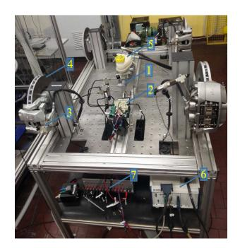
Figure 3.19 HIL Test Rig 1-TMC 2-customized ESC 3-Brake caliper 4-Brake disk 5-oil tank 6-Data Acquisition System 7-Relay Box
