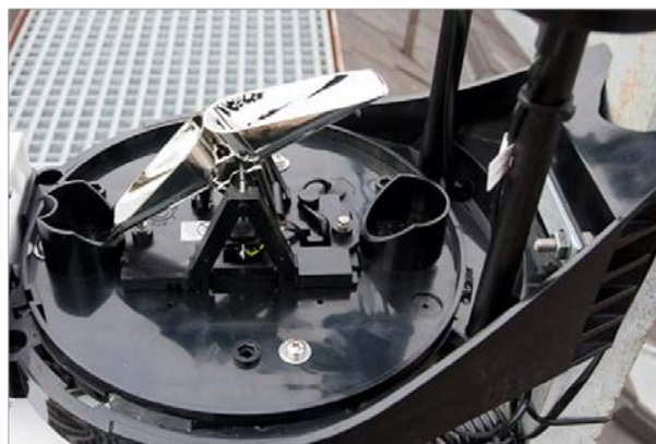
Figure 2.2 - Internal trays of a Davis tipping bucket rain gauge
