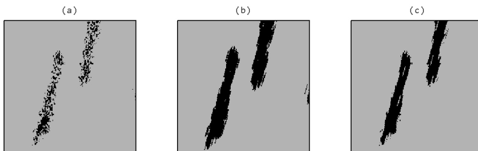
Figure 4.7 - (a) Original mask made from S_1=5 . (b) Filtered mask with large directional filter with l=15 pixels. (c) The previous picture after application of an erosion filter of the same size
