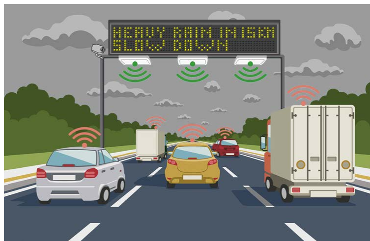
Figure 6.4 - The surveillance cameras detect rain and send a message to the (connected) cars. The users can adapt their driving behaviour in advance, avoiding crashes and casualties
