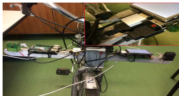
Figure 4. Bike mobile system with all sensors installed
