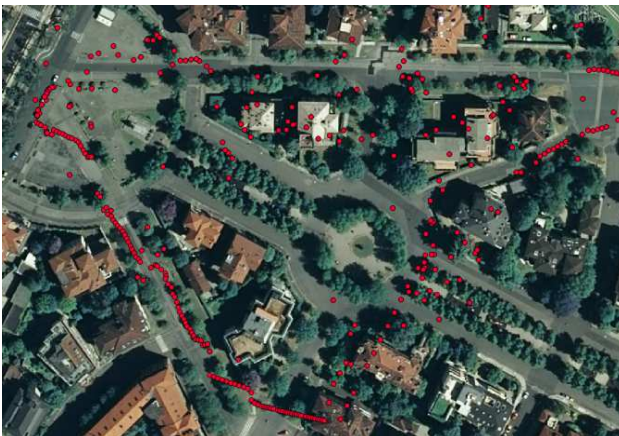
Figure 13. Camera positions measured by the GNSS device.
