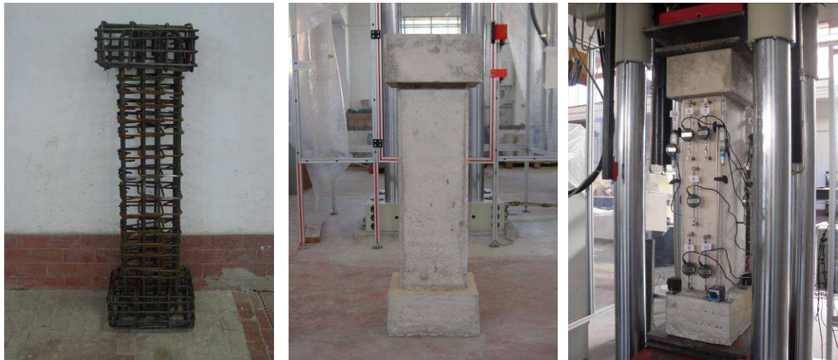
Figure 2.1. Arrangement of reinforcement, specimen and specimen under test
