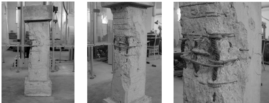
Figure 4.4. Specimen CEY2 after test
