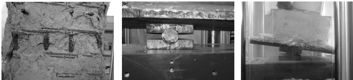
Figure 4.6. Ultimate state of specimen CEX1; rotation of device at the top and base of specimens
