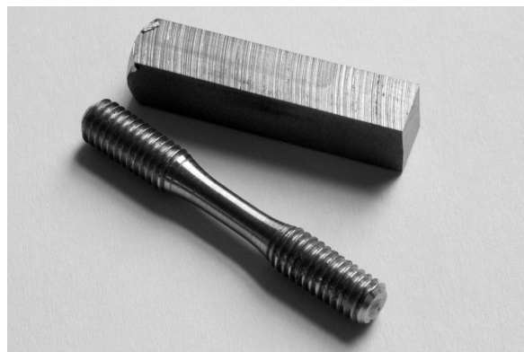
Fig. 3.1 Prismatic sample 7x7 mm cross section and sample after turning.
