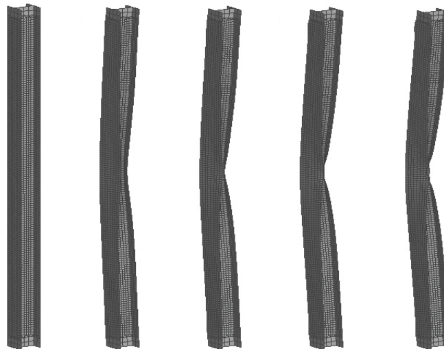
Fig. 6.15 Frames acquired during a numerical simulation (FF, 20kg of eq. TNT at 1 m and 550°C).
