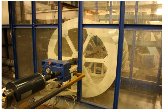
Fig. 4.2. The investigated overshot water wheel, with diameter 1.46 m and width 1 m.
