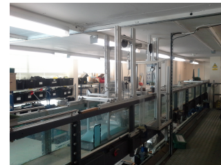
Fig. 5.1. The test channel. (a) The water depths were measured at 1 (for the weir), 2 and 3 (upstream and downstream water depth, respectively); (b) a picture of the Flume.
