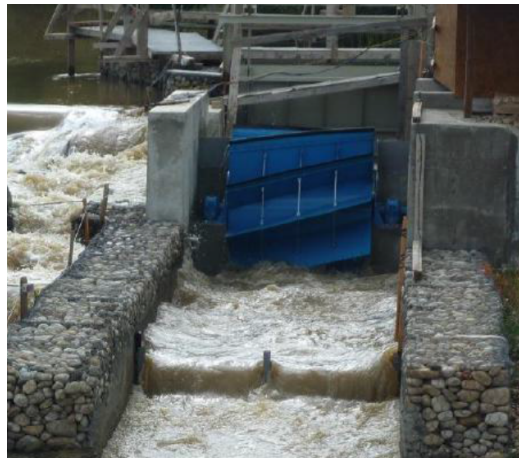
Fig. 1.11. The Hydrostatic Pressure Machine (Bozhinova et al., 2012).
