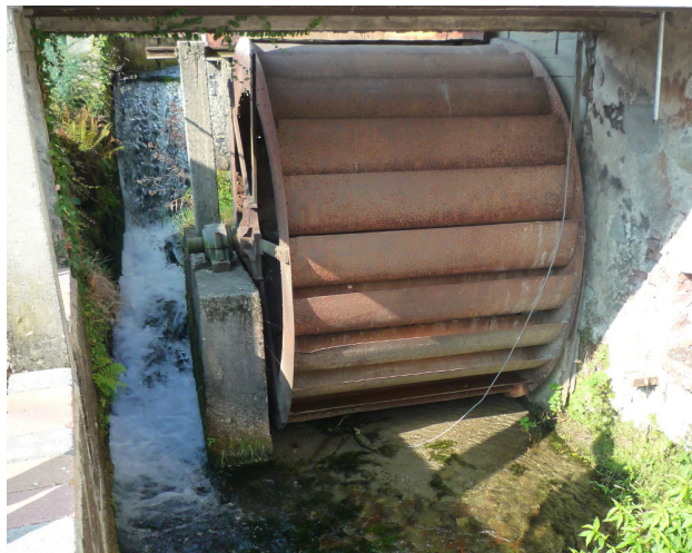
Fig. 4.1. The overshot water wheel in Ciconio, with diameter 3 m and width 2 m.
