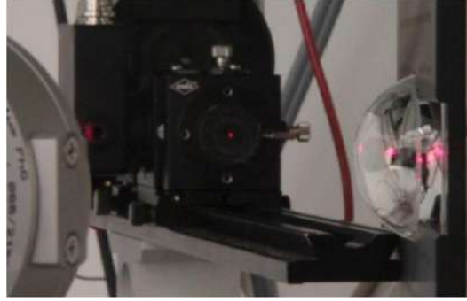
Fig. 2.8 Goniometer set-up comprising half ball lens coupling for large observation angles.
