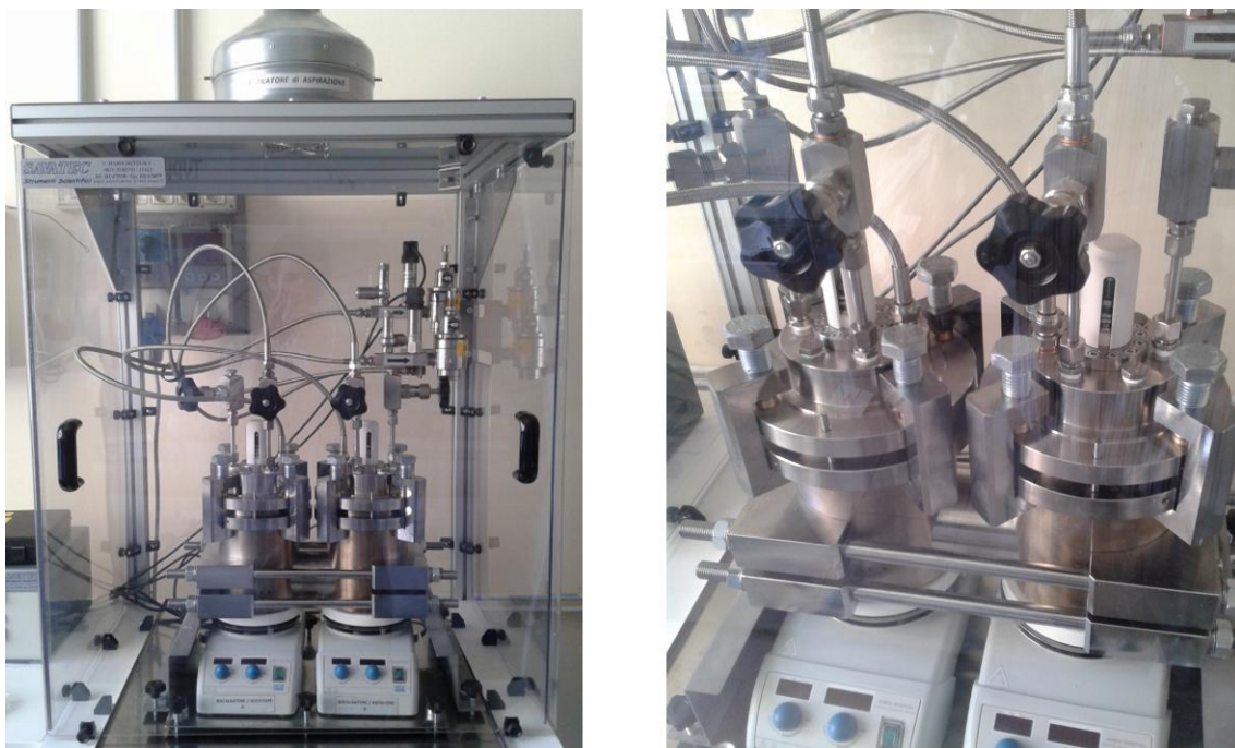
Fig. 75 – Reactor used for the High-Temperature High-Pressure (HTHP) tests
