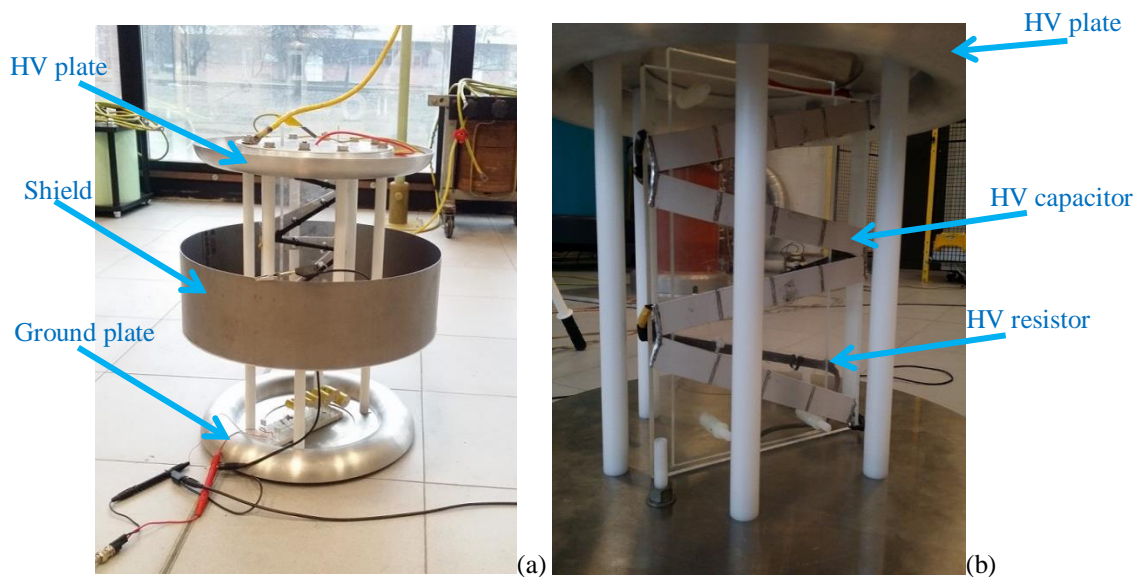
Fig. 3.138. Realized RCVD (a) general view (b) HV part (shield is not shown here)
