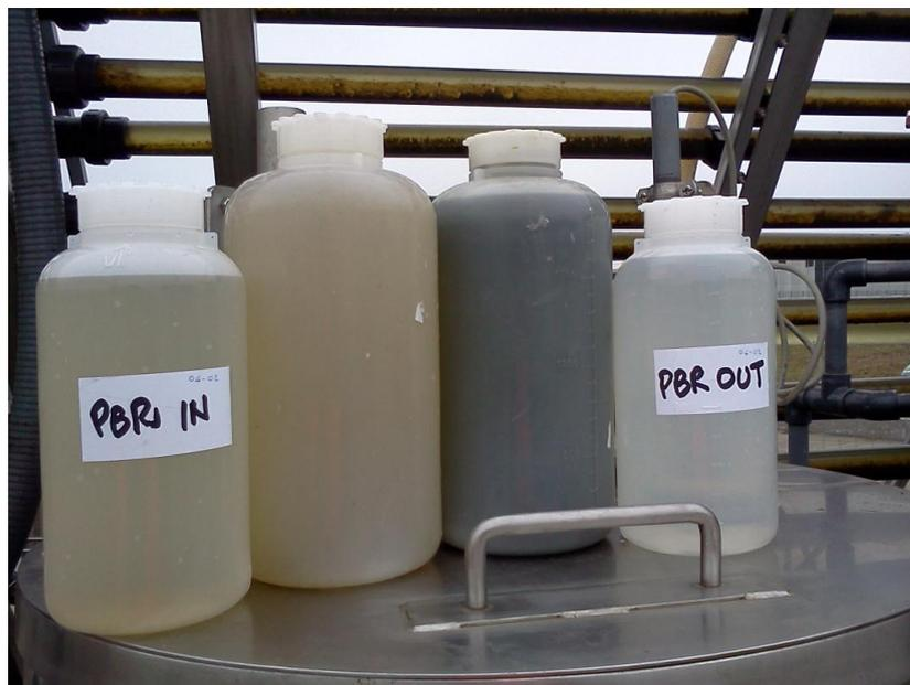
Figure 76. From the left to the right hand. Samplings: 1. PBR inlet water. 2. Water recirculating in the PBR. 3. Algae attached to the pipe. 4. PBR outlet water.
