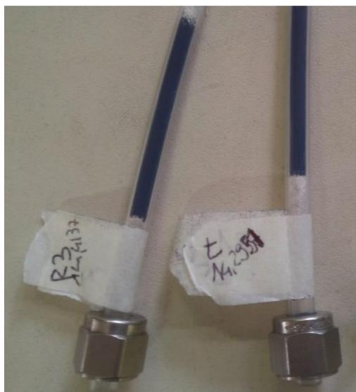
Figure 188. Micro-reactors for AC testing.
