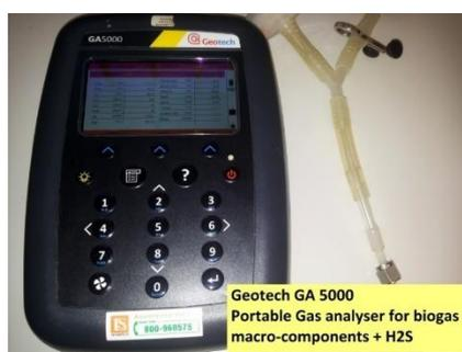
Figure 233. Geotech gas analyzer.
