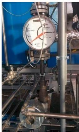
Figure 54. Air blower and its Rotameter
