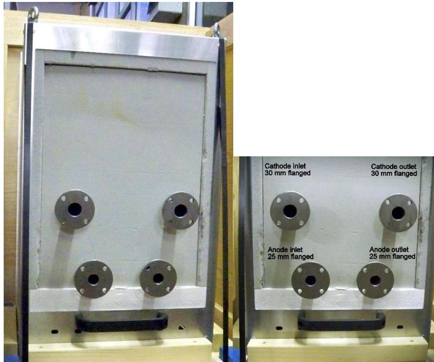
Figure 51. SOFC stack, with the four manifold (anode in/out, cathode in/out). Electrical connections where places at the other side of the box.
