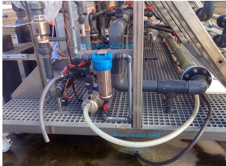
Figure 68. Inlet wastewater flow to the system.
