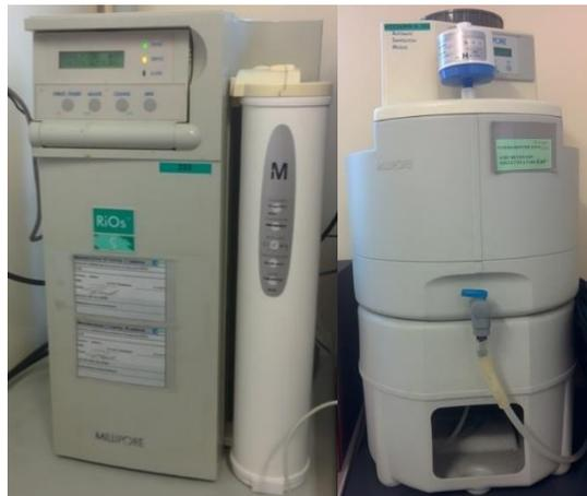
Figure 46. Tap water demineralizer RioS 5 + 30 L tank
