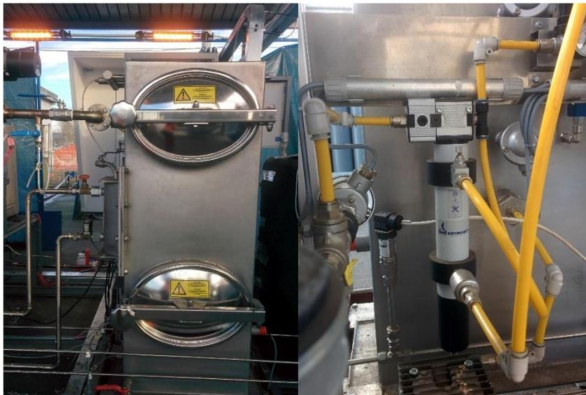
Figure 63. Condenser (on the left) and CO<sub>2</sub> separation membrane (on the right).
