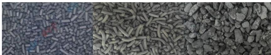
Figure 187. Activated carbons: from left to right hand: Airdep ACs, Sulfatrap R7E, Sulfatrap R8G.
