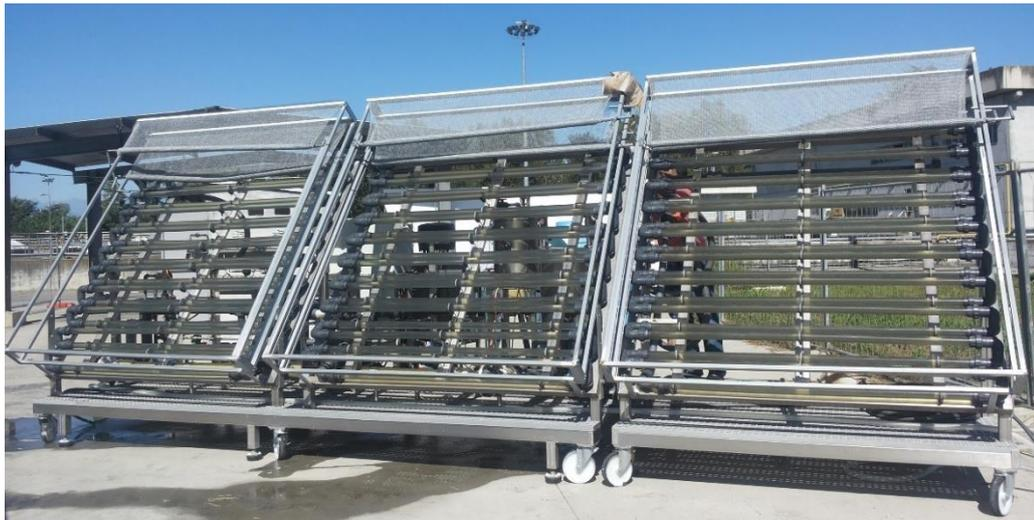
Figure 40. SOFCOM proof-of-concept at the SMAT Castiglione WWTP –CO<sub>2</sub> utilization for algae growth.
