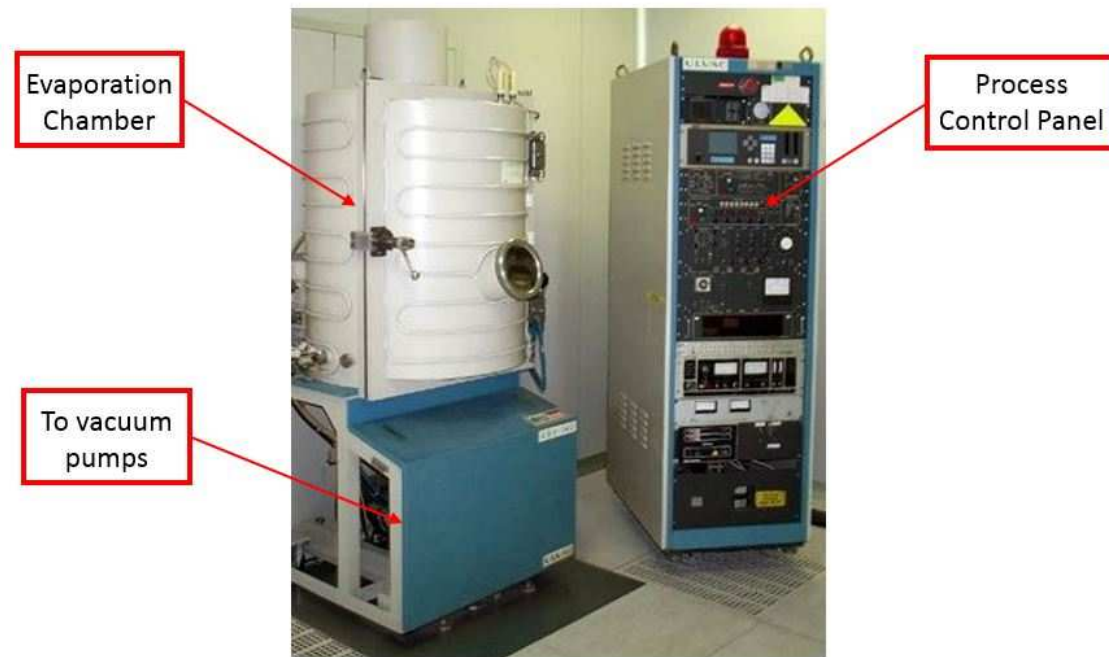
Fig. 3.18 E-beam evaporator ULVAC EBX-14D system available at Material and Microsystems Laboratory (Chilab) of the Politecnico di Torino, in Chivasso (TO) [34].
