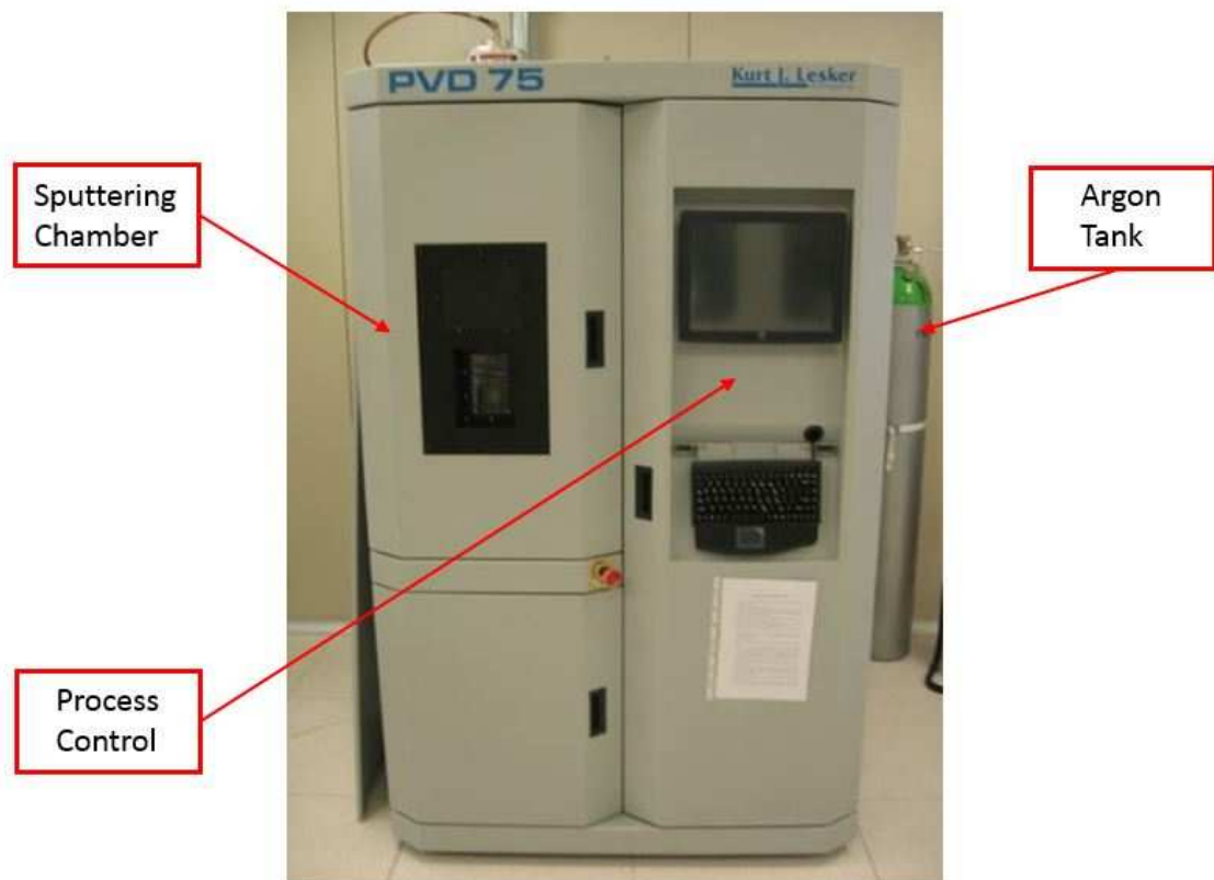
Fig. 3.2 Commercial RF magnetron sputtering system PVD 75 (Kurt J. Lesker Company, England) available at TechFab, Chivasso (TO) used for silicon dioxide deposition [5].
