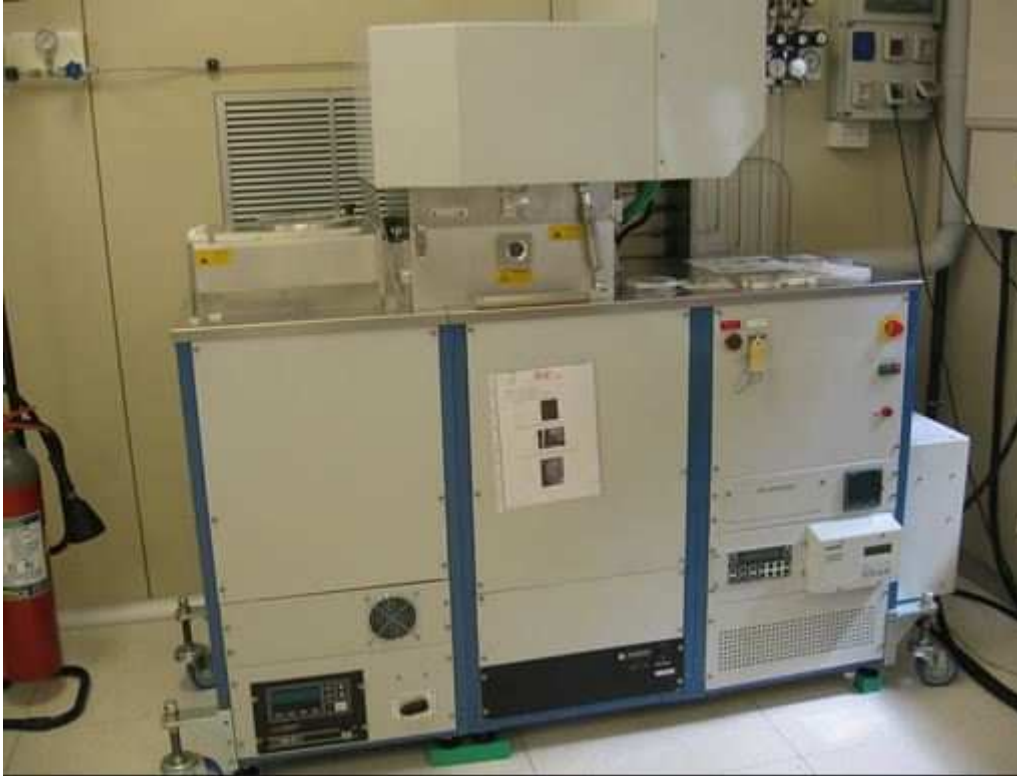
Fig. 3.13 ICP-DRIE Oxford Plasmalab 100 system available at TechFab, Chivasso (TO) used for both silicon dioxide and silicon plasma etching [20].
