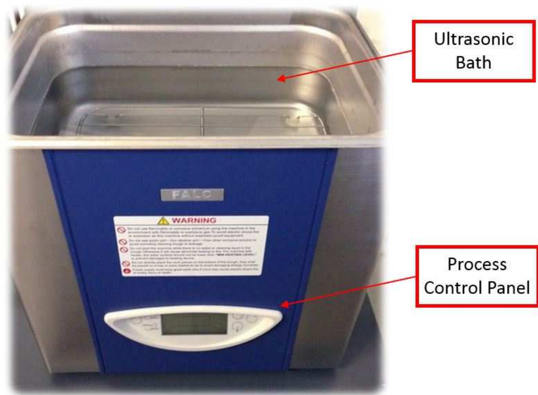
Fig. 3.21 Labsonic LBS2 -15 system available at Material and Microsystems Laboratory (Chilab) of the Politecnico di Torino, in Chivasso (TO) [36].
