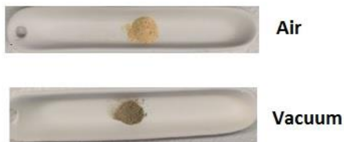
Figure 4-8: The Fe-0.7-MeIMO-DS powder sample, treated in air and vacuum at 500 °C, for 4 h with the heating rate of 5 °C.min -1
