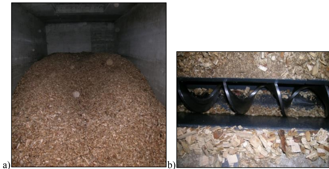
Figure 5.1 – Chips storage (a) and screw conveyor system (b)
