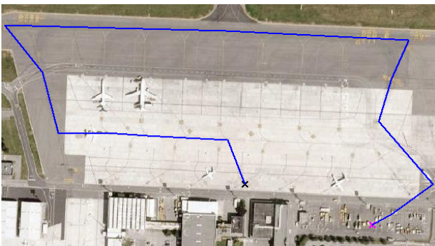
Figure 19: Algorithm 3. Departure mission, Phase 1: from tractor deposit to departing aircraft parking lot. Credits: Pictures 2015 DigitalGlobe, Map data ©2015 Google.
