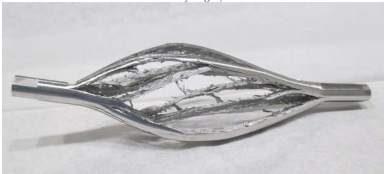
Fig. 1: Damage induced in Iridium rod as a consequence of high energy proton beam impact (the beam is coaxial with the rod and hits the rod at the centre of one base) during the HRMT27 experiment, in which equivalent conditions as the ones reached in the AD-target core were recreated [7, 9].
