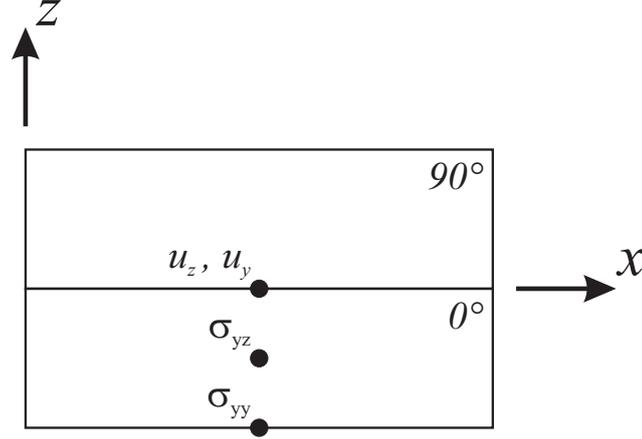
Figure 4: Cross-section and verification points of the two-layer asymmetric cross-ply beam.
