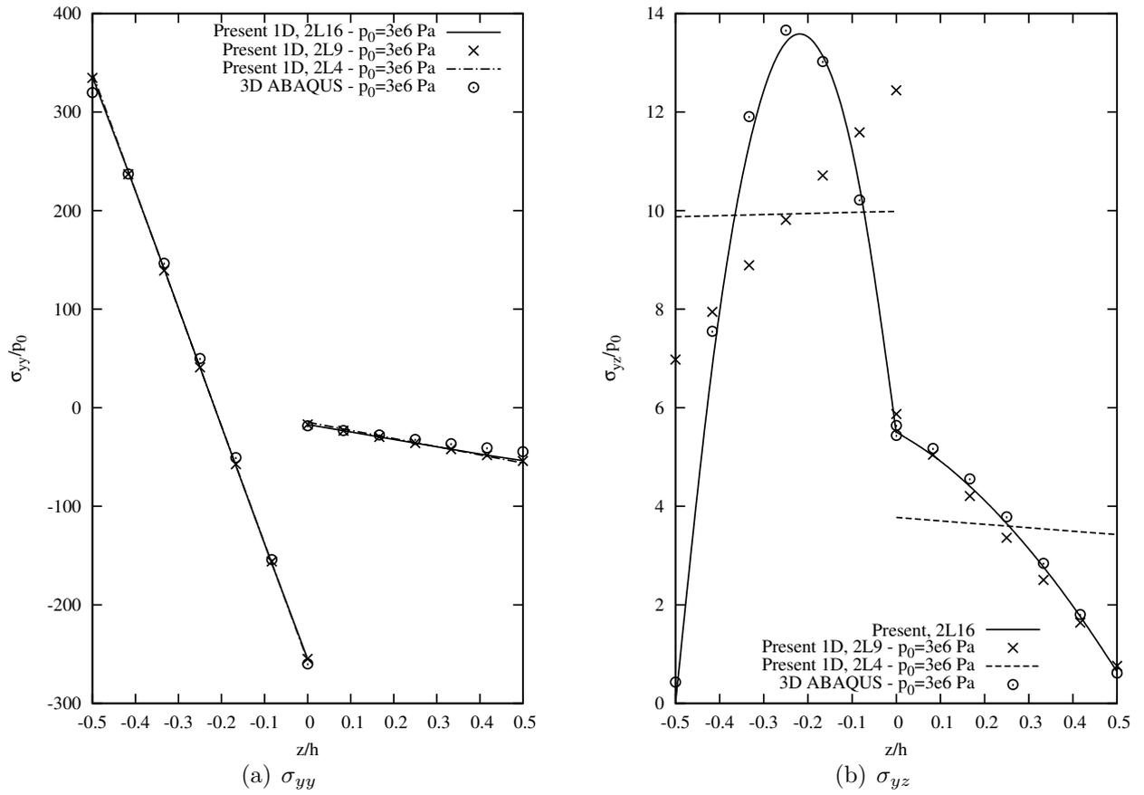
Figure 7: Through-the-thickness distribution of axial,  $\sigma_{yy}$ , and transverse,  $\sigma_{yz}$ , stress components at the mid-span of the cantilever asymmetric cross-ply beam subjected to bending. Nonlinear analysis,  $p_0 = 3 \times 10^6$  Pa.
