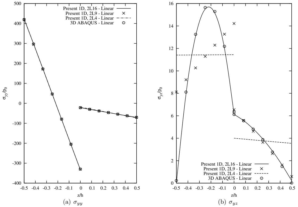
Figure 6: Through-the-thickness distribution of axial,  $\sigma_{yy}$ , and transverse,  $\sigma_{yz}$ , stress components at the mid-span of the cantilever asymmetric cross-ply beam subjected to bending. Linear analysis.
