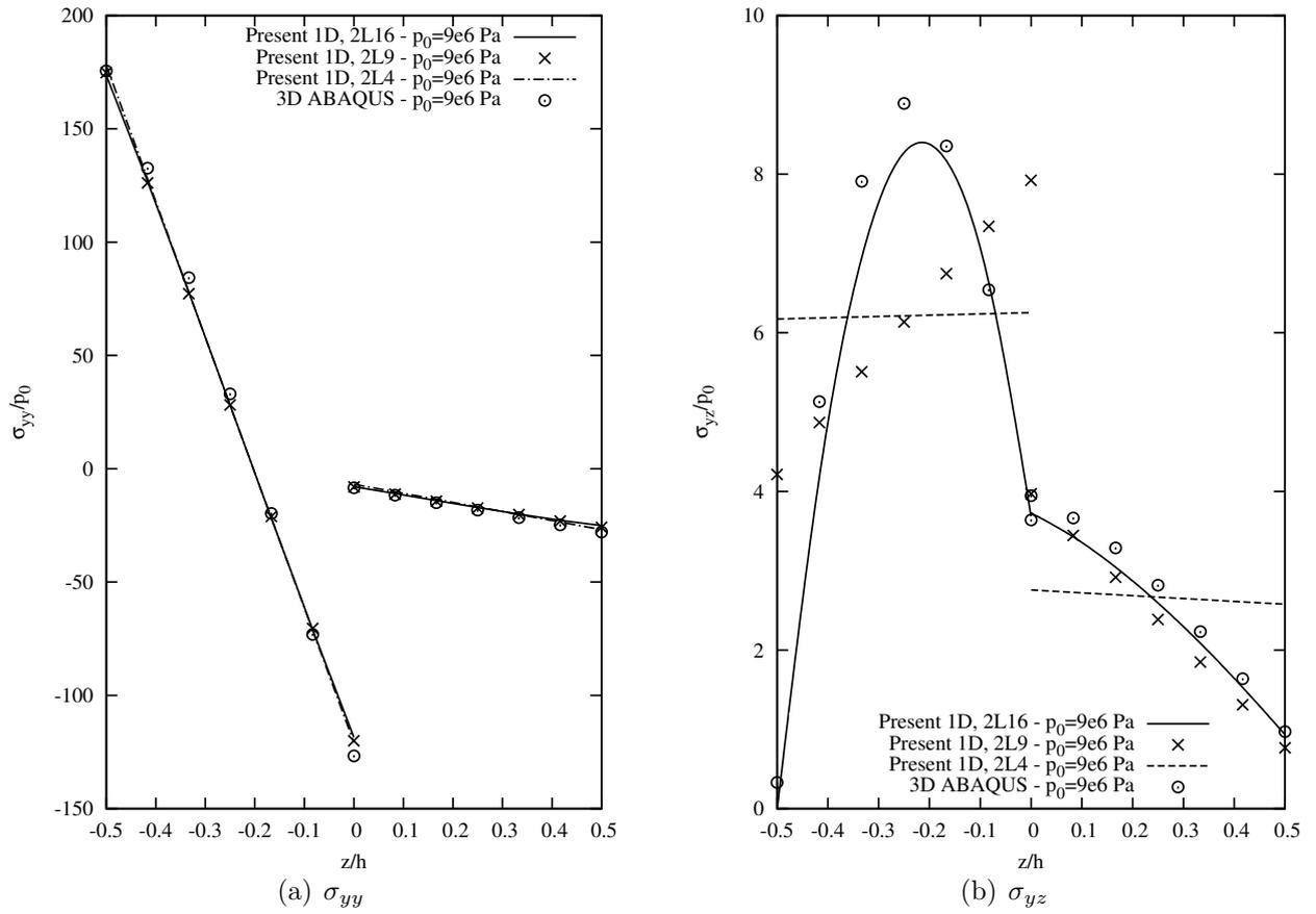
Figure 8: Through-the-thickness distribution of axial,  $\sigma_{yy}$ , and transverse,  $\sigma_{yz}$ , stress components at the mid-span of the cantilever asymmetric cross-ply beam subjected to bending. Nonlinear analysis,  $p_0 = 9 \times 10^6$  Pa.
