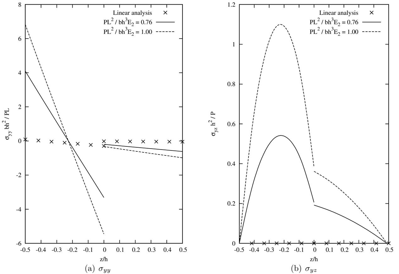
Figure 11: Through-the-thickness distribution of axial,  $\sigma_{yy}$ , and transverse,  $\sigma_{yz}$ , stress components within linear and geometrical nonlinear ranges.  $[0^\circ/45^\circ]$  composite beam subjected to compression and clamped-free boundary conditions. 2L16 beam model.
