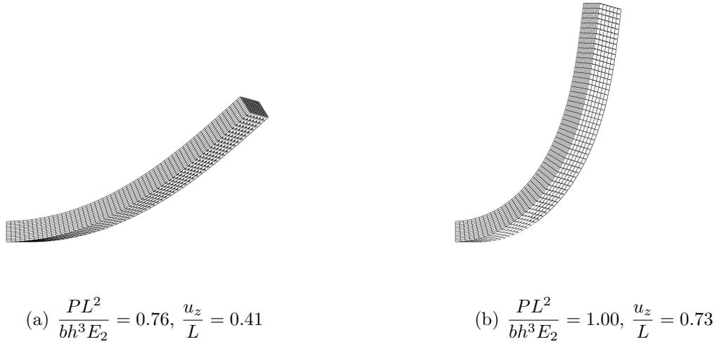
Figure 10: Three-dimensional displacement views of the cantilever  $[0^\circ/45^\circ]$  composite beam subjected to compression. 2L16 beam model.
