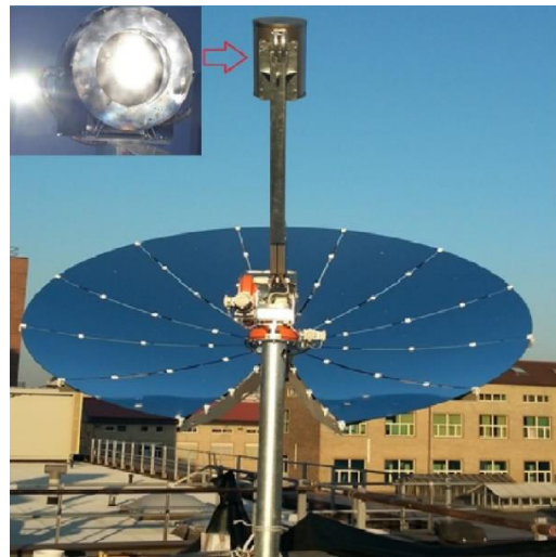
Fig. 2. Picture of the solar concentrator installed at Politecnico di Torino (Turin, Italy). The receiver is depicted in the zoom inset.
