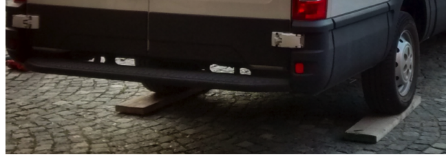
Figure 8.19: Positioning of the vehicle on the wooden base for the emulation of a the condition of transmitter at 5 cm under the ground level.
