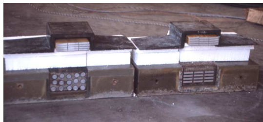
Figure 2.4: Cross-section of the buried transmitter and the on board receiver of the PATH prototype.
