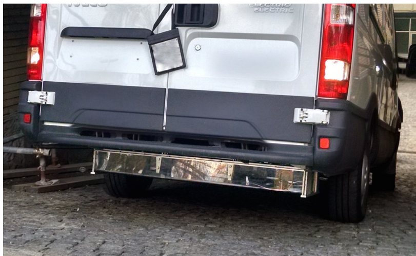
Figure 6.20: Receiver structure mounted under the vehicle.
