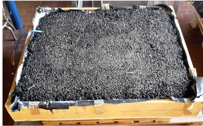
Figure 7.12: Last layer of cold asphalt for the tests on coil A.
