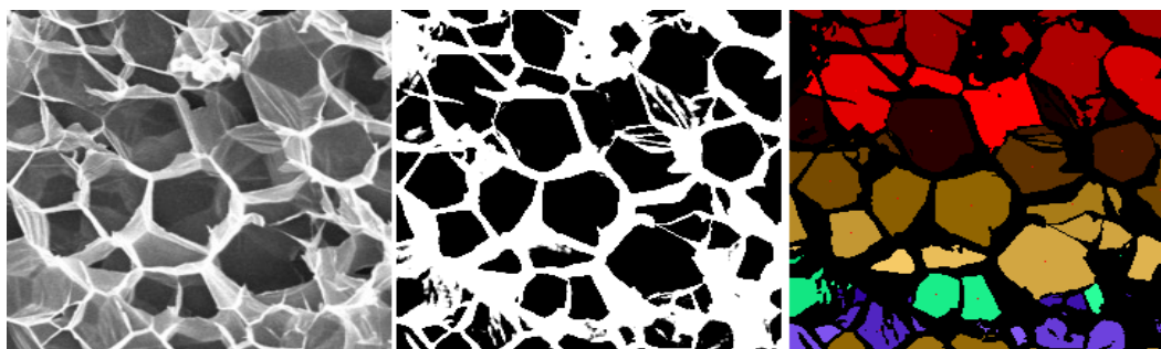
Figure 8: The grey-tone image (240 x 240 pixels) is given in the left panel (Microcellular Plastic Micrograph developed at Indian Institute of Technology, Delhi. Courtesy: Gandhi.iitdelhi, Wikipedia). In the middle, the corresponding black and white image obtained after a thresholding. On the right, the result of the segmentation is given. Each super-pixel is rendered in different colour tone.
