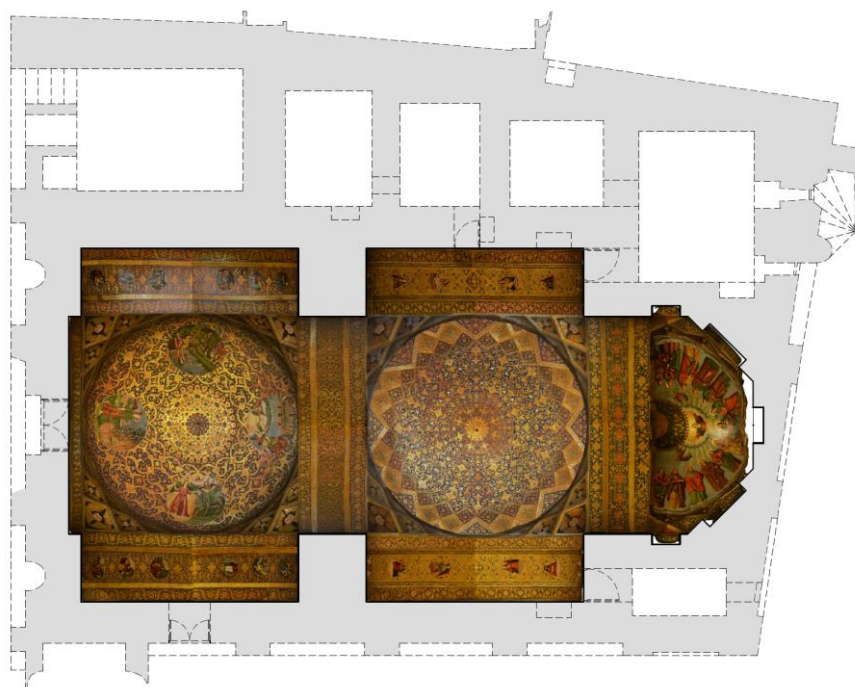
Figure 6. The complete vaults orthoprojections superimposed on the upwards plan.
