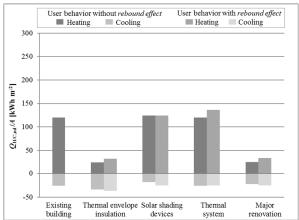
**Figure 2:** Net energy need for heating and cooling normalized by the heated floor area 6 User 1
