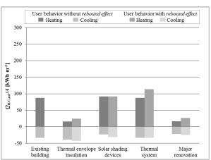
**Figure 4:** Net energy need for heating and cooling normalized by the heated floor area 6 User 2
