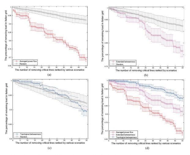
Fig. 2. Remaining load in the Italian power grid after removing 50 most critical lines in various scenarios. (a) Random attack versus power flow criterion attack. (b) Random attack versus extended betweenness criterion attack. (c) Random attack versus topological betweenness criterion attack. (d) Comparison between the three criteria.
