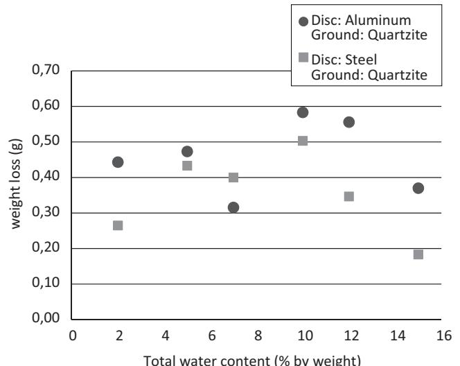
Fig. 3. Loss weight diagram for quartz sand conditioned with different percentage of water obtained by using aluminum and steel discs.
