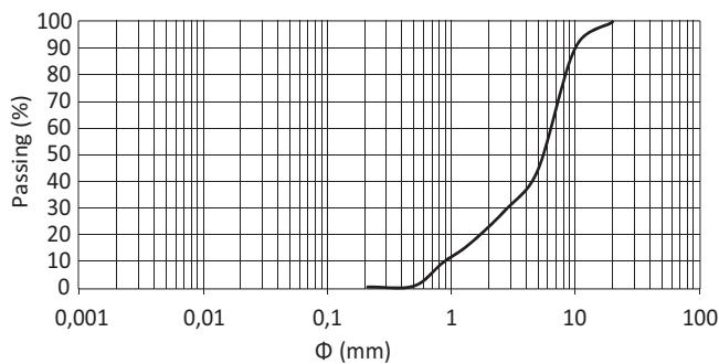
Fig. 2. Grain size distribution of the used quartz sand.
