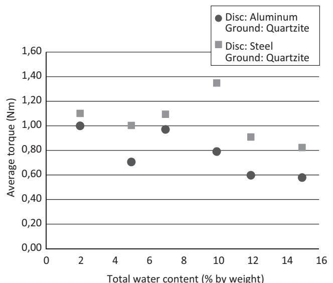
Fig. 4. Torque diagram for quartz sand conditioned with different percentage of water obtained by using aluminum and steel discs.
