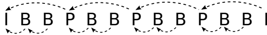
Fig. 2 Concealment algorithm te_1 : reference frames used in case of loss for a typical GOP pattern.
