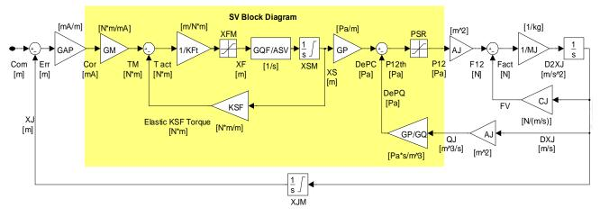
Fig. 3: Block diagram of the EHA mathematical model used for the prognostic algorithm
