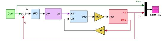
Fig. 2: Simulink block diagram of the considered EHA.
