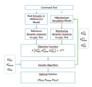
Fig. 4: schematic of the proposed FDI procedure.
