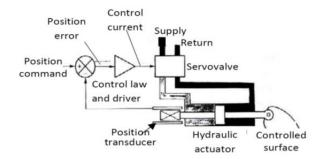
Fig. 1: Concept schematic of the EHA actuator
