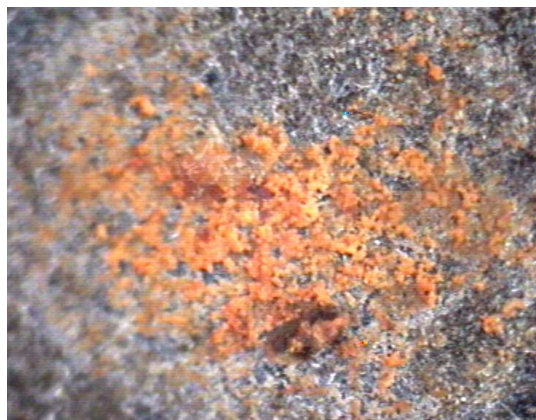
Fig.4 General corrosion on a AISI 309 component (800X magnification)
