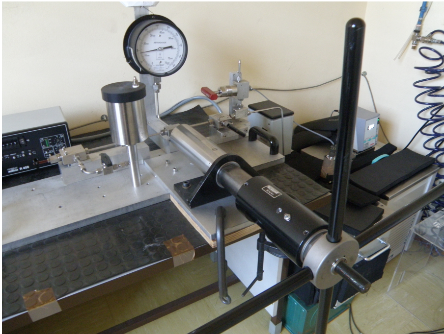
Figure 2.11: Picture of the high-pressure circuit and the pressure amplifier.
