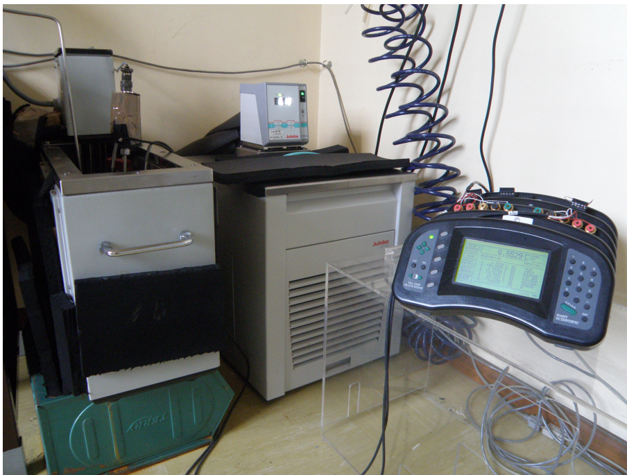
Figure 2.12: Picture of the temperature control system.
