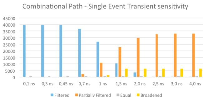
Figure 4. Combinational Path-Single Event Transient Sensitivity.
