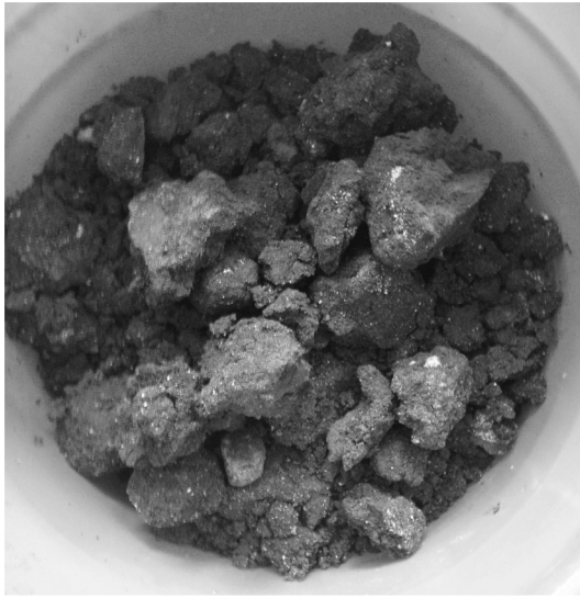
Fig. 1. Picture of the soil tested in the laboratory. It is possible to see the sand aggregated in blocky elements.
